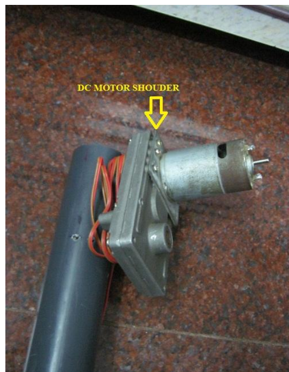
Fig. 3.5: DC Motor in the shoulder
