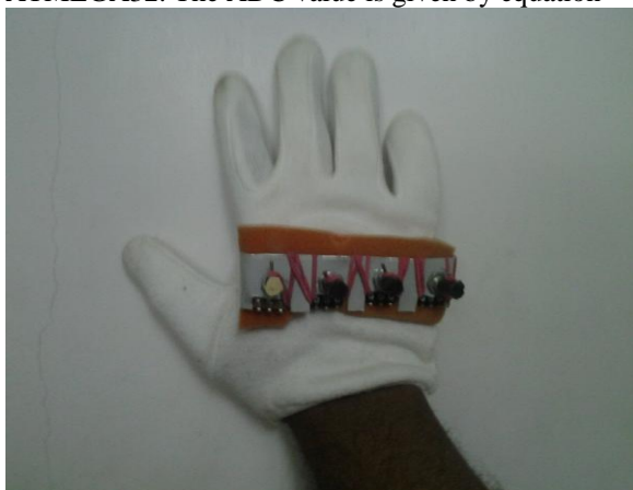
Fig 3.1: Mounting of potentiometer on Hand glove
