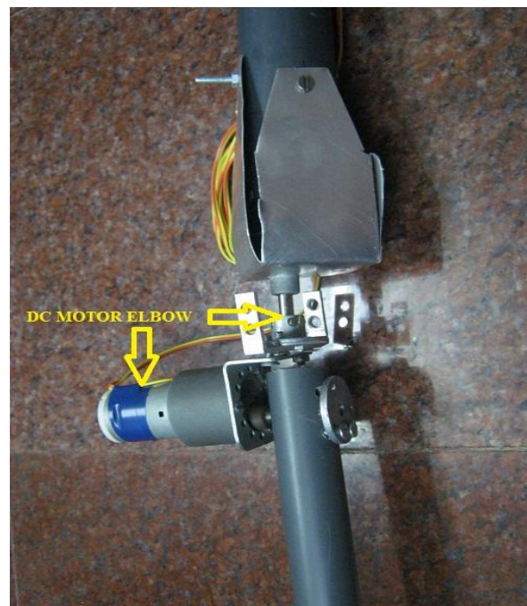
Fig. 3.4: DC Motors in the elbow
